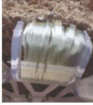
Fig. 5: Microspine toe securely gripping and hanging from a rocky surface [14].
