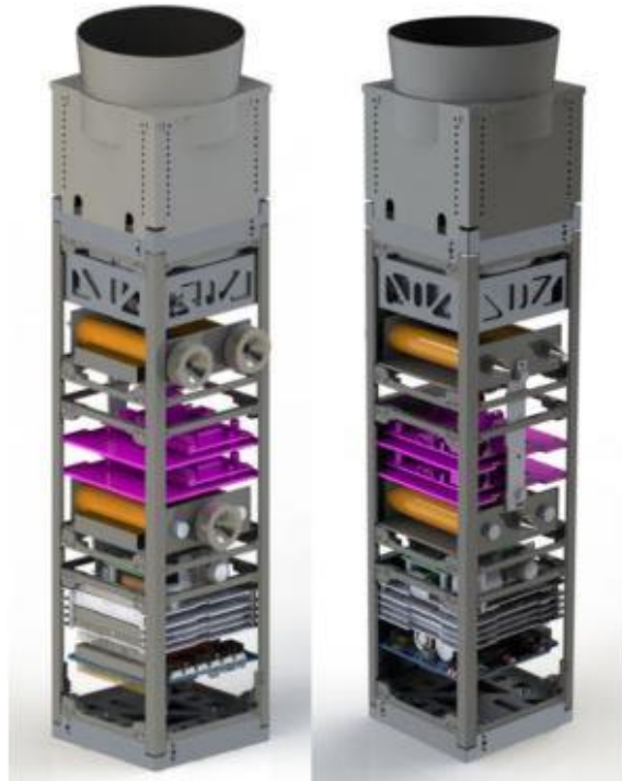
Figure 4: MirrorSats of the AAReST Mission (courtesy of [8]).
