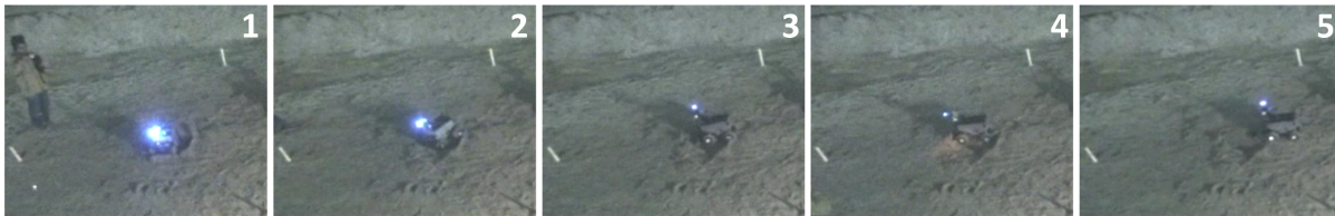
Figure 4.18: Video snapshots of rocking behaviour followed by a ‘backout’ behaviour triggered after the rover gets stuck trying to push the blade forward.
