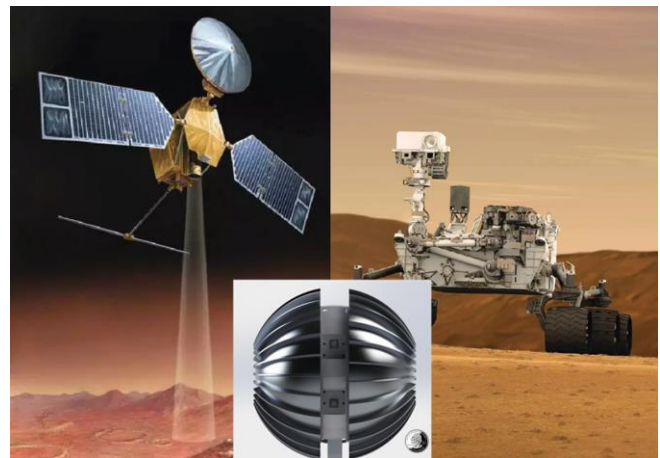
Figure 1: Spherical, cantaloupe sized robots (inset) can be deployed from large rovers such as the Mars Science Laboratory and access rugged terrains too risky to traverse by large rovers or be visible to orbital assets such as Mars Reconnaissance Orbiter.
