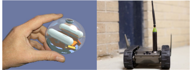
Fig. 1. Example of small robots (Left) A ball shaped hopping robot concept for exploration of extreme terrains and caves developed for NASA. (Right) iRobot 110 Firstlook used for observation, security and search and rescue.
