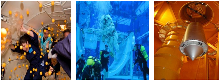
Figure 1. Methods to simulate low-gravity conditions include use of parabolic flight (left), neutral buoyancy in large water tanks (center) and use of drop towers (right).
