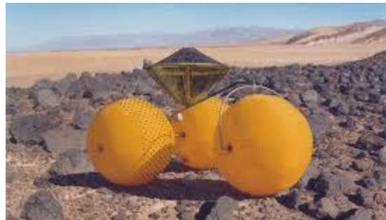
Figure 1: JPL's Inflatable rover concept traversing rugged planetary environment.
