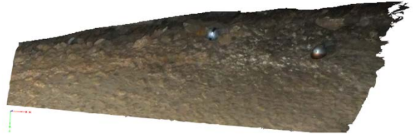
Fig. 7- Stereo images taken to produce 3D point cloud and mesh images of the pit-bots inside a lava tube (Flagstaff, Arizona).
