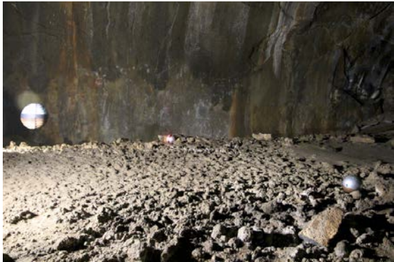
Fig. 5- A network of 3 ball robots in a lava tube (1 flying mockup consists of a quad copter). Two on the ground are static display. Our studies show that the flying robot can locate/identify other robots within a 7 m distance.
